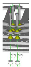
Using the 4-40 x 5/8" socket head cap screws (x4), brass cone washers (x4) and large 4-40 lock-nuts (x4), attach the links to the lower arm. Slide the screws through the captured ball ends then through the cone washers, then thread them into the holes closest to the center of the chassis. Keeping a hex driver in the screw, use a nut driver to install the 4-40 nuts from below the chassis. The screws should be held snug to the carbon lower arm when tightening the nuts.
