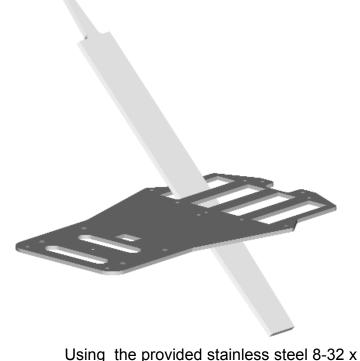
Using the provided stainless steel 8-32 x 1/2" cross point (phillips) screws (x4), attach the lower front suspension arm (be sure the pockets for the pivots are facing down. The screws will thread into the holes shown. Be sure to keep the plate as even as possible, tightening opposite screws a little at a time equally. This will ensure that attaching these two plates together will not introduce any tweak into the chassis. Do not over tighten.
